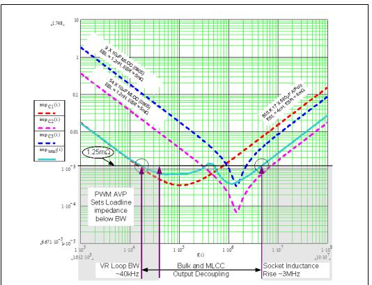
Figure A-2. Z(f) Network Plot with 1.25  $m\Omega$  Load Line
